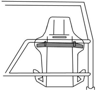
If the seat sits behind the b/pillar hoop a secondary support to the cage must be added. An example of this is shown in the diagrams within this section of the document. If the modification goes to the floor it must be sat on 23cm square plate 3mm (min.) thick.
